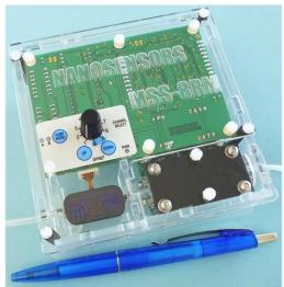
MSS 8 Channel Readout Module (MSS-8RM) is a basic electronic module to operate and to readout NANOSENSORS™ MSS, up to 8 sensors simultaneously, under a hardware configuration for electronic nose/odor sensing. MSS-8RM contains two air pumps and users can examine self-prepared MSS under different gas flow conditions.
