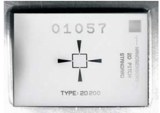
Photograph of a 2-dimensional pitch standard showing a 200 nm pitch at the center area.
