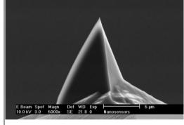
AFM Tip: Phosphorus doped Silicon
