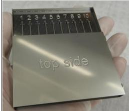
NANOSENSORS™ developed a box fabricated solely from metal avoiding the usage of adhesion gel and plastics.
