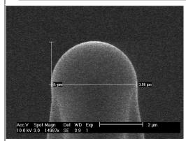
AFM Tips: Silicon / Silicon Oxide. Different versions are available:
