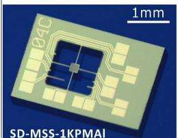
**Working Principle:** A sample attached to the platform tends to align with the applied magnetic field, which twists the torsional axis and bends the bending axis on which piezoresisors are embedded. By measuring the resistance change, the magnitude of the yielded force can be estimated.
