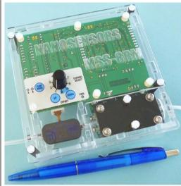
MSS 8 Channel Readout Module (MSS-8RM) is a basic electronic module to operate and to readout NANOSENSORS™ MSS, up to 8 sensors simultaneously, under a hardware configuration for electronic nose/odor sensing. MSS-8RM contains two air pumps and users can examine self-prepared MSS under different gas flow conditions.
