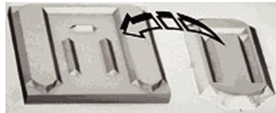
SEM-Picture of Alignment Chip and Backside of POINTPROBE® Holder
