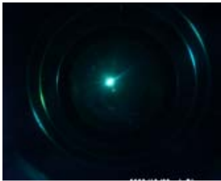
Video image of the field emission (emitter voltage: 70 V)
